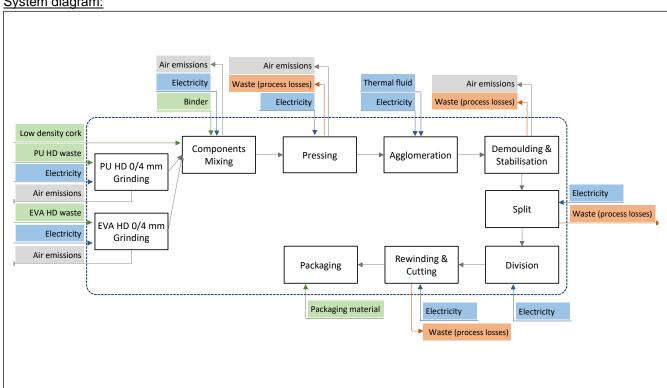
The Underscreed U36 production comprises 11 stages: Low density Cork Grinding (outside ACC facilities), PU HD 0/4 mm Grinding, EVA HD 0/4 mm Grinding, Components Mixing, Pressing, Agglomeration, Demoulding & Stabilisation, Split, Division, Rewinding & Cutting and Packaging.
